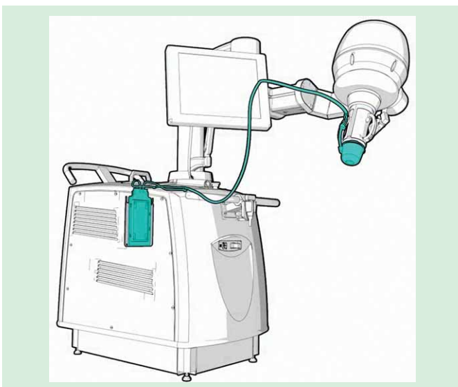
Figure 2. Device's set-up used to remove air bubble from the circulating water and enable consequent wave transmission and skin protection during the treatment.
